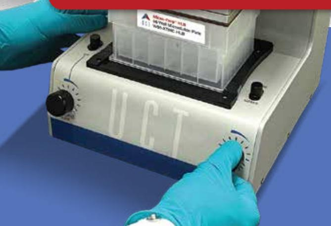
Micro-Prep™ MMCX with mixed-mode cation exchange functionality extracts polar and non-polar analytes from aqueous samples.
